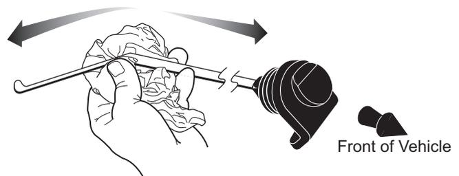
The oil should be checked with the engine warm. The vehicle should be on a level surface with the parking brake engaged. Allow adequate time for oil to drain into the crankcase before checking.
