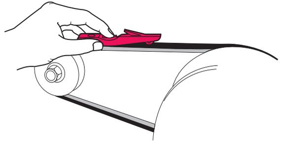
Tighten an existing belt to 75 - 80 lbs. (34 - 36 kg) tension using the same technique and inspect for cracking or wear. A maximum deflection of 1/2" (13 mm) is acceptable.
