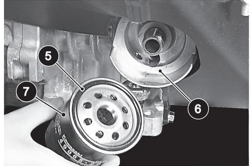
Inspect the new oil filter for any defects. Apply clean engine oil to the oil filter O-ring (5) and install the oil filter onto the engine until the seal contacts the mounting surface. Turn the filter 2/3 to 3/4 turn by HAND. Pour in the specified type and amount of oil. See CAPACITIES AND REPLACEMENT PARTS.
