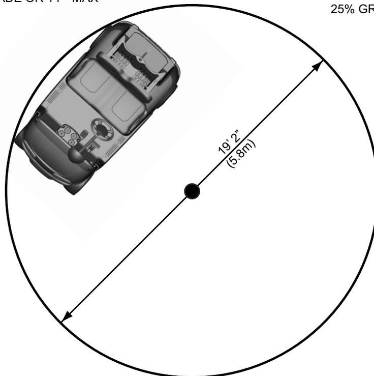
Figure 3 Vehicle Incline Specifications and Turning Diameter
