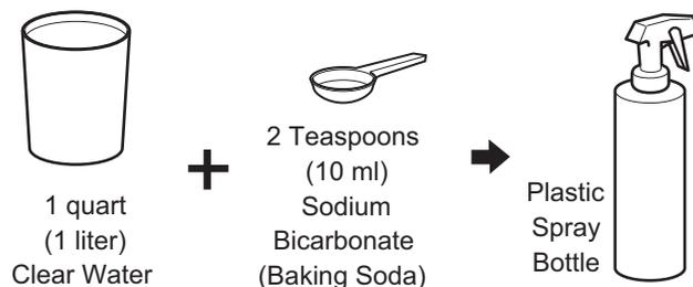
The correct cleaning method is to spray the top and sides of the battery with a solution of baking soda and water. Apply this solution with a plastic spray bottle. The solution is 2 teaspoons (10 ml) sodium bicarbonate (baking soda) mixed with 1 quart (1 liter) of water. Spray the solution on all metal components near the battery also.
