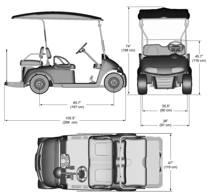
Figure 2 Shuttle 2 + 2 Vehicle Dimensions
