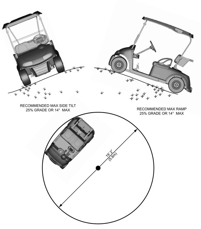
Figure 3 Vehicle Incline Specifications and Turning Diameter
