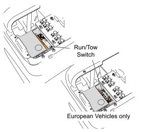
Figure 3 Run/Tow Switch
