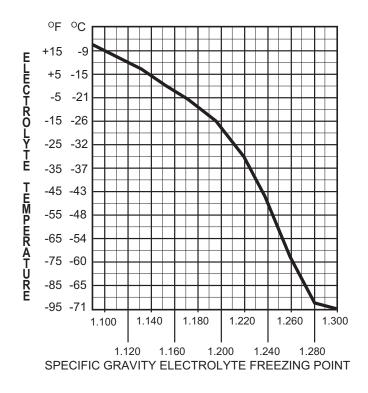
Figure 9 Freezing point of electrolyte
