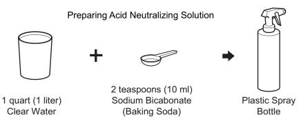
The correct cleaning method is to spray the top and sides of the batteries with a solution of baking soda and water. Apply this solution with a plastic spray bottle. The solution is 2 teaspoons (10 ml) sodium bicarbonate (baking soda) mixed with 1 quart (1 liter) of water. Spray the solution on all metal components near the batteries also.
