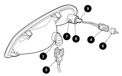
Figure 1 Headlight and Turn signal bulb replacement
