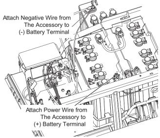
Figure 2 Accessory Wires to Battery Pack
