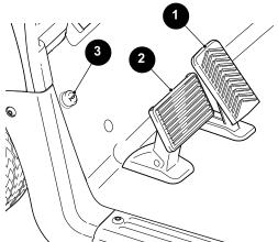
Figure 2 Accelerator and Brake Pedal Operation
