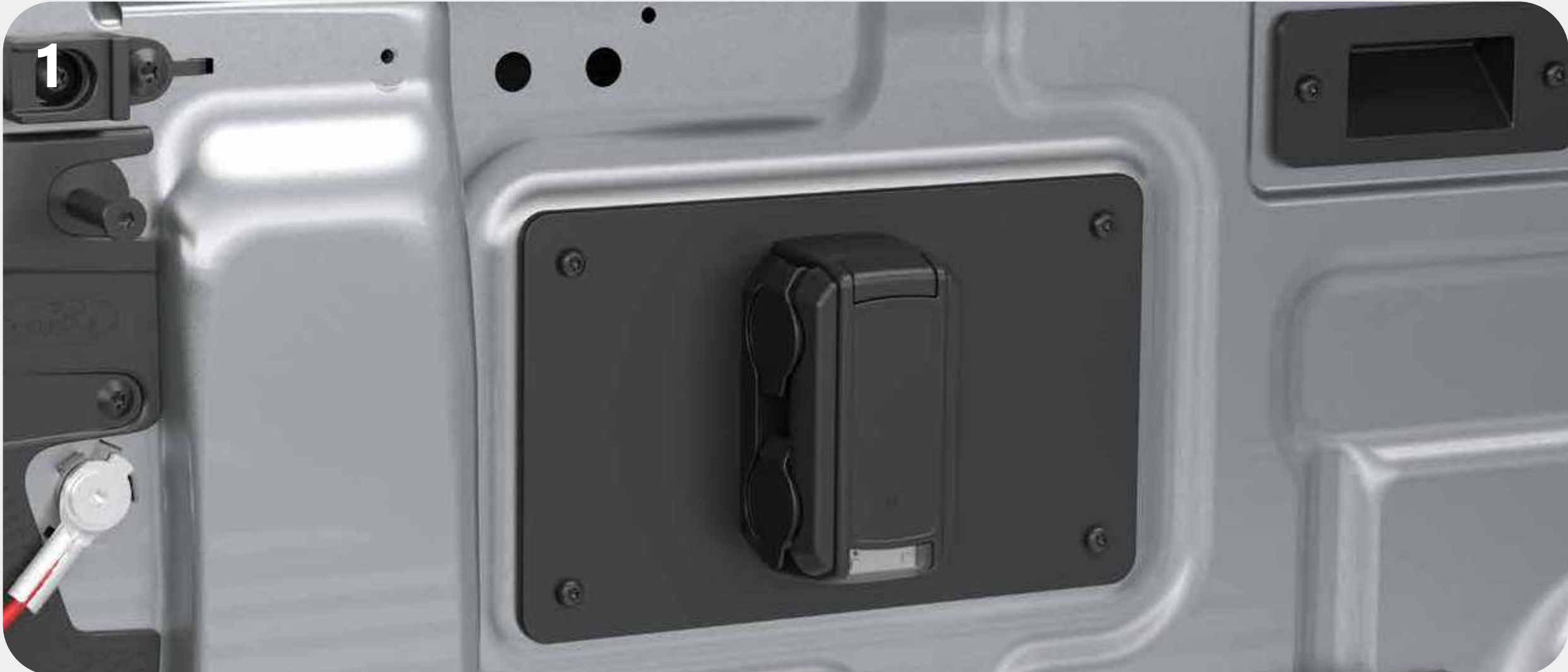
1 Auxiliary 12V Smart Power Outlet - Dual Socket with Light All Variants without factory power outlets in the load box
