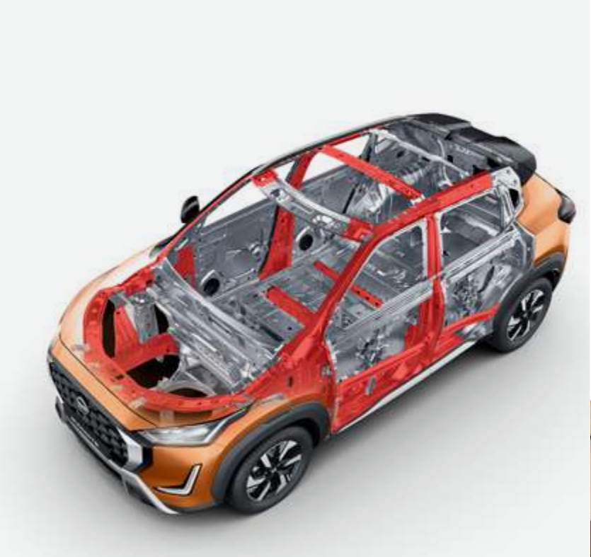
67% Usage Of High Tensile Strength Steel
