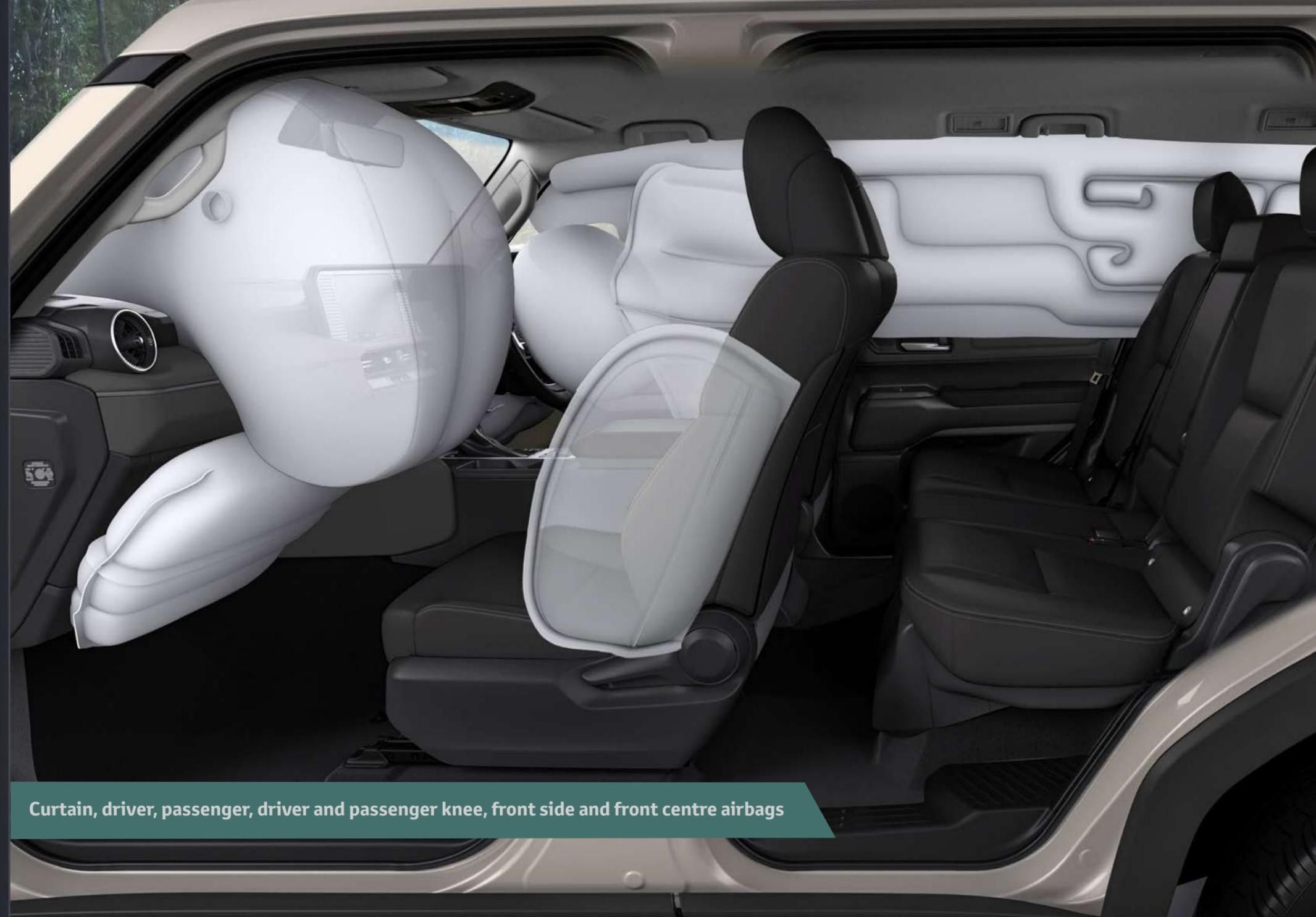
Curtain, driver, passenger, driver and passenger knee, front side and front centre airbags
